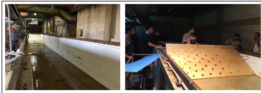
Figure 2: CAMERI wave flume with demountable texture plate.
