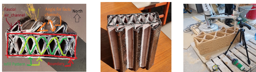
Figure 3. Images from left to right - (a) Crossing section of wall component, (b) Glazed ceramic object, shading effect is visible, (c) Final Print, reaching 40cm height
