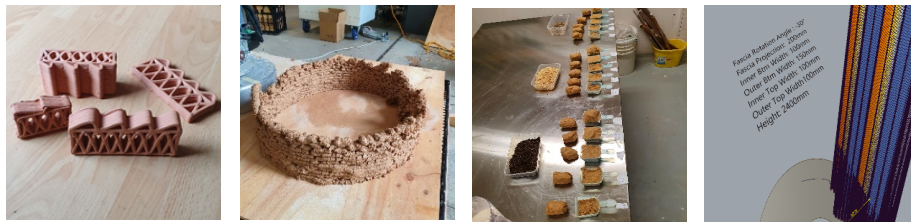
Figure 2. Images from left to right - (a) Sample 3d printed ceramics with various parameters value, (b) Failed print, not having a suitable viscosity, (c) Systematic material mixing, (d) Result of radiation analysis used in geometry optimisation
