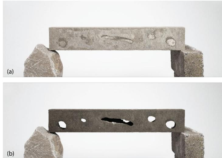
Figure 7. Case study 2 result. (a) Before gypsum support is removed. (b) After gypsum support is removed.
