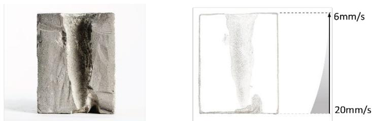
Figure 3. Cavity size according to the gradual printing speed change.
