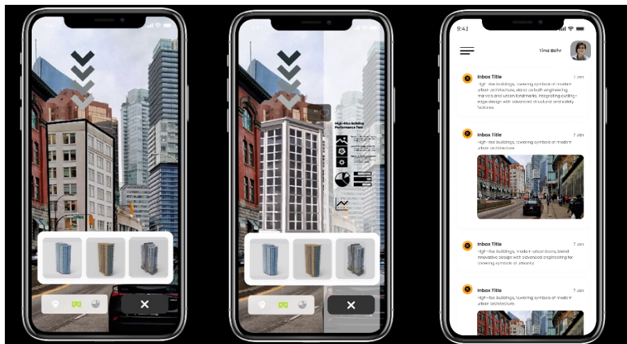
Figure 3. An In-situ virtual view of a design proposal can be viewed from different angles (left), while an on-demand view of relevant data summary can be shown as expandable data visualization (centre). The stakeholders can share their comments on a social-media thread in D-ARE (right).
