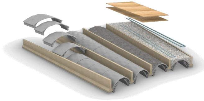
Figure 1. Exploded Axonometric of the 3dcp hybrid slab, showing assembly of elements
