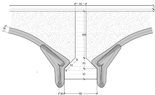
Figure 2. Detail section of slab design
