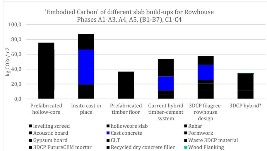
Figure 3. Embodied carbon of different slab build-ups based on standard Danish construction specifications for a rowhouse typology
