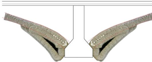
*Figure 4. Diagram showing the wrapping of print paths*
