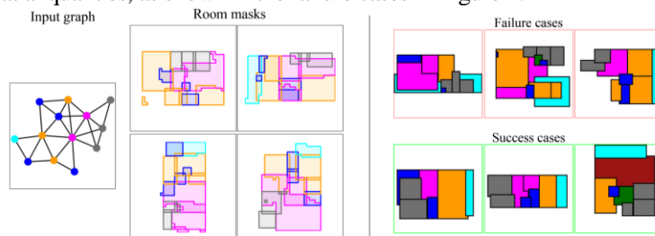
Figure 2. Left: Overlapping bounding boxes of rooms in House GAN. Right: Failure and success examples of the generation (source: Nauata et al., 2020).
