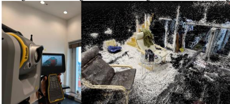
Figure 2 Indoor space scanning with Trimble SX12
