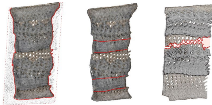
Figure 4. Left: boundary difference showing receding impact. Centre: Clustering of the overhang layer showing loss of definition, Right: boundary proximity for detection of cracks and missing parts
