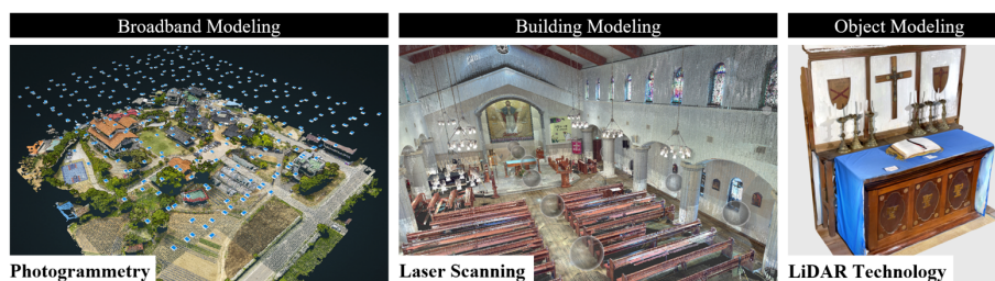
Figure 6. 3D Modeling techniques through the use of photogrammetry, laser scanning, and LiDAR
