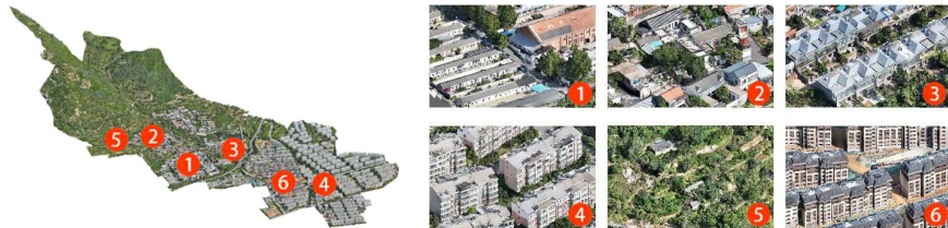
Figure 3. 3D model of Baimashi Village generated by UAV photos and DJI Terra
