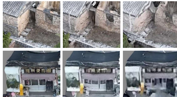
Figure 1. The first row of images from left to right: Aerial Photogrammetry in 45m, 90m and 135m above the ground, showing building materials; The second row of images from left to right: Aerial Photogrammetry in 45m, 90m and 135m above the ground, showing store sign
