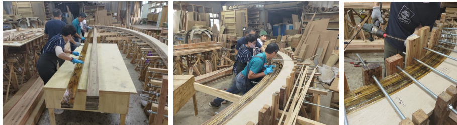
Figure 7. a) Manual application of polyurethane adhesive, b) Layers of Japanese cedar are manually pressed into the jig, c) High-pressure vices are used to clamp the geometry
