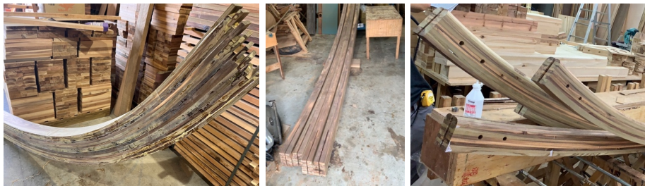
Figure 8. a) Ring beam prior to sanding, b) Ring beams with steel plate slots, c) Catenary beams with rounded top profile
