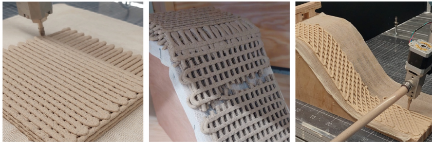
Figure 5-7 (left to right). 3D Orthogonal pattern printing, Non-planar orthogonal print failure, Non-planar weaving pattern printing
