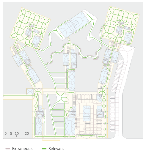
Figure 1. Medial Axis Transform (MAT) graph: Extraneous edges that will not be used are in grey and edges to be used for analysis are in green.
