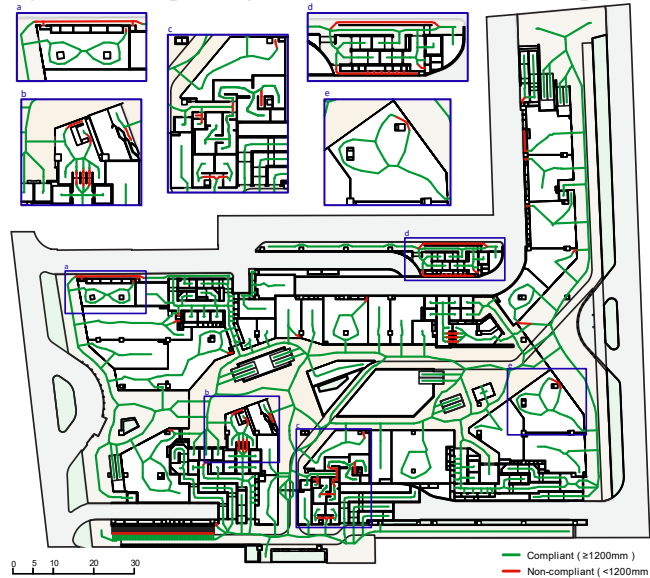
Figure 3. Checking for corridor compliance
