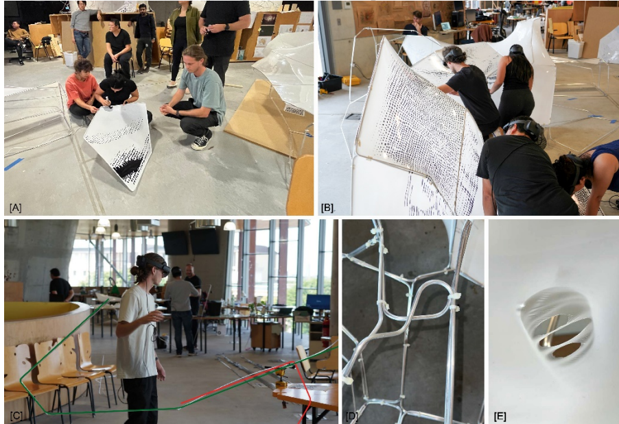
Figure 4. [A] Developing drawing techniques. [B] Collaborative drawing session. [C] Evidence of students reframing problems from learning ‘bad fit’ with AR. The red line indicates a clash between the pipe geometry and the desk. [D] Geometric constraints of pipe-bender on a consecutive tight radius. [E] Overheating of shrink film during the wrapping process.
