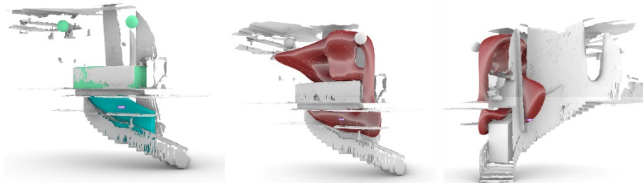
Figure 3. On the top left is a 3D scan of the stairwell using HoloLens; the cyan-coloured objects identified physical constraints. Centre and Right, design proposal for a structure that would sit on the balustrade and form around the concrete stairwell.
